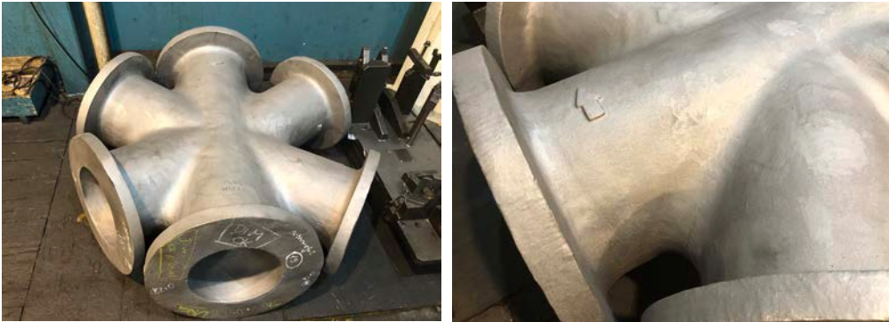
Figure A.4 Cast node (left). ‘Up’ indicators were cast into the nodes to aid rapid assembly (right)
