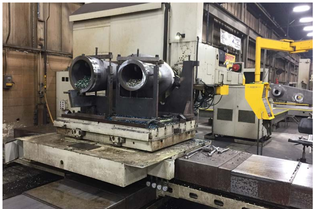
Figure A.12 CNC machining of casting to facilitate fit-up with incoming columns
