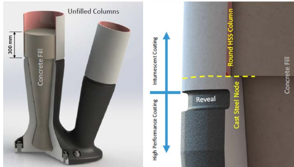
Figure A.11 The cast base achieved two hour fire resistance by increasing the wall thickness and infilling with concrete
