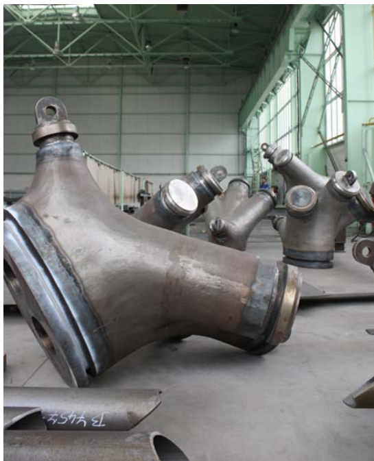
Figure A.2 Steel castings at the fabrication shop
